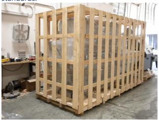
18. Your PP-5545TBD Automatic L' Sealer comes fully crated and bolted to a heavy duty fully enclosed pallet to protect your machine during shipment.
